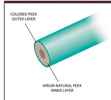
Our dual layer PEEK tubing eliminates any concern that a critical sample stream could be contaminated by pigments used to color code the tubing. It looks like any other color-coded tubing at first glance, but a closer look reveals that the pigmented layer\* surrounds a separate but integrally-bonded inner layer of natural PEEK. Only natural PEEK is in contact with the fluid stream.
