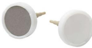
The Last Drop mobile phase filter allows more analyses per batch of mobile phase and helps reduce hazardous waste. The flat filter element sits parallel to the bottom of the reservoir, allowing the Last Drop to filter all but the last 2% of the mobile phase from the reservoir without drawing air into the system. Compare this with conventional cylindrical filters that can begin to draw air into the system when nearly 10% of the solvent remains in the reservoir.
