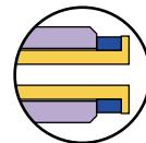
For those systems requiring or preferring flanged connections, use these fiberglass-reinforced fittings with our Easy-Flange flanging tool and polypropylene washers to make a clean connection. The flange on the tubing ensures that the washer never comes in contact with the mobile phase.
