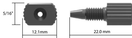
For tightening tool, use either a ValvTool (JR-800, page 102) or an open end wrench (JR-804, page 103.)
